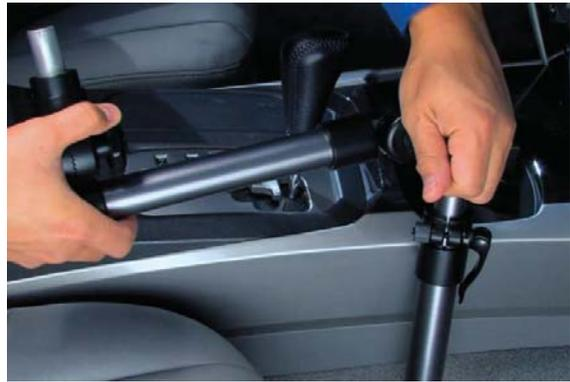
6. Place the plastic deck on the top of the aluminum stand and then plug in and tighten the handle.
