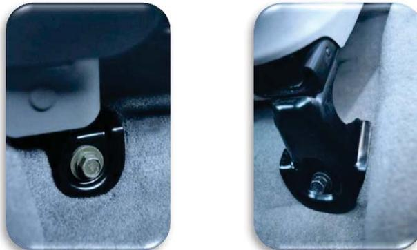
3. Mounting base options: There are several options to set up your mounting base. Please find the setup option that best fits the seat bolt and seat rail design under the front left corner of your passenger seat.
