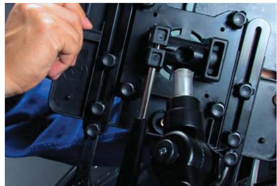
7. Set your device on the deck and adjust the four sliding supports (two in the front and two in the back).
