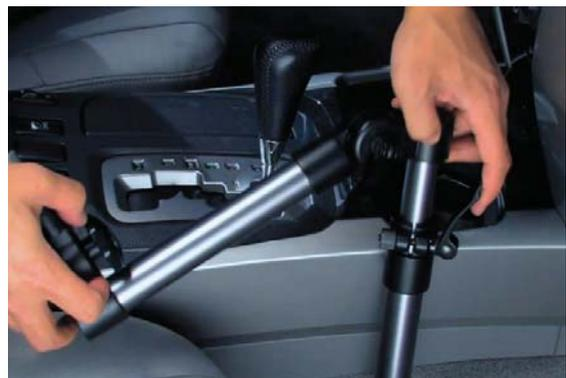
5. Loosen the lever on the teeth-locking joint and adjust the angle of the upper tube. When finished, tighten the lever.
